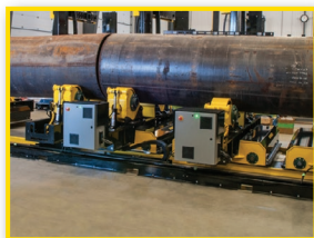
Sections brought together using powered track drive.
