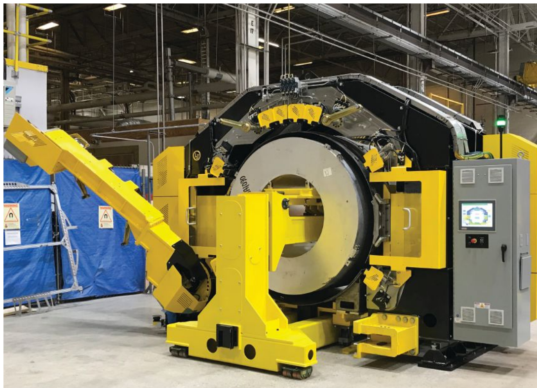
Edmonton-based LJ Welding Automation installed a universal rounding station at GE Healthcare's South Carolina plant. The 28-axis forming device corrects parts that have minor inconsistencies.
