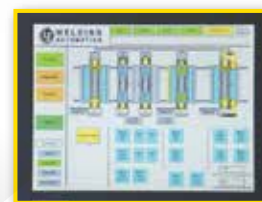
Easy to use HMI touchscreen to control hydraulic jacking, alignment, indexing/track drive, and powered rotation
