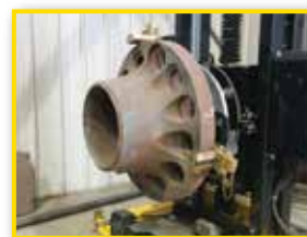
Optional Tailstock system available for adding flanges or end caps
