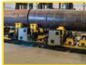
Sections brought together using powered track drive
