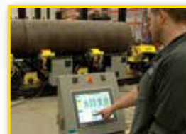
Variable speed and bidirectional controls for rotation, alignment, leveling and/or rail mount drive
