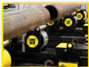
Pipe loaded, lined up using track drive
