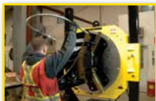
Remove hold down u-bolt
