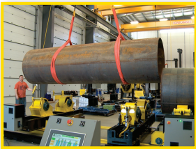
Each section loaded onto rolls.
