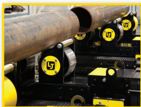
Pipe loaded, lined up using track drive.
