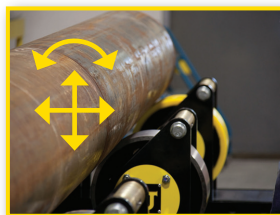
Alignment, side shift, and leveling functionality.
