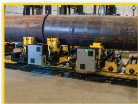
Sections brought together using powered track drive.
