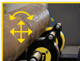
Alignment, side shift, and leveling functionality.
