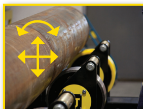
Alignment, side shift, and leveling functionality.
