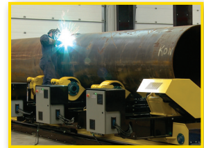
Ready for fit up and/or automated welding, then index for next section to be added.
