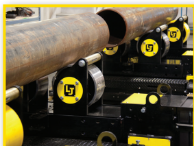
Pipe loaded, lined up using track drive.
