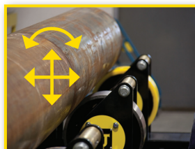
Alignment, side shift, and leveling functionality.
