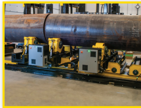
Sections brought together using powered track drive.
