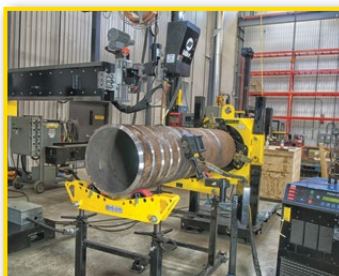
Optional fully integrated rolling induction heating systems.
