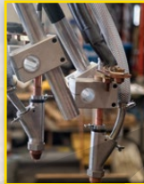
Double SAW custom weld head set-ups
